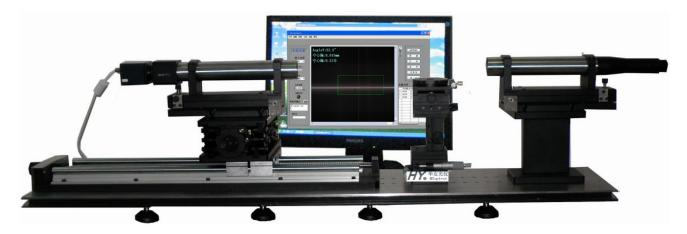
LensCT-HTR is a high precision eccentricity tester designed for Cylinder Lens and Rectangular shape spherical Lens. The horizontal layout could allow the testing lens stand on station with the datum surface and prevent the polished surfaces for any damage. It includes both Transmission and reflection mode testing, and could be used for perpendicularity, parallelism and output beam deviation testing as well.
