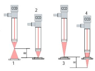
As per the definition, the RoC means the travel distance of 1&2 or 3&4.
