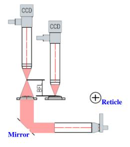
The software will automatically calculate the EFL of tested sample based on the double slit image, and will show the result directly.
